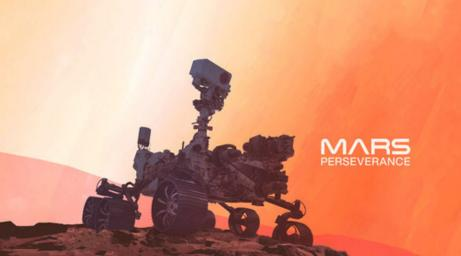
The Mars 2020 Perseverance Rover will search for signs of ancient microbial life, which will advance NASA's quest to explore the past habitability of Mars. The rover has a drill to collect core samples of Martian rock and soil, then store them in sealed tubes for pickup by a future mission that would ferry them back to Farth for detailed technologies to help pave the way Mars.
