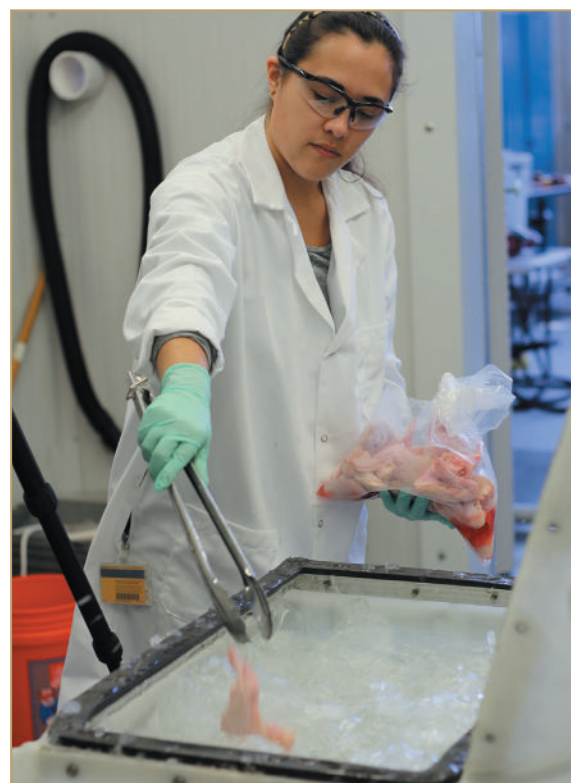
Stephanie Richter, graduate research assistant, uses a GTRI-designed micro-chiller to test ice slurry's antimicrobial capability for chicken parts (wings) chilling.
